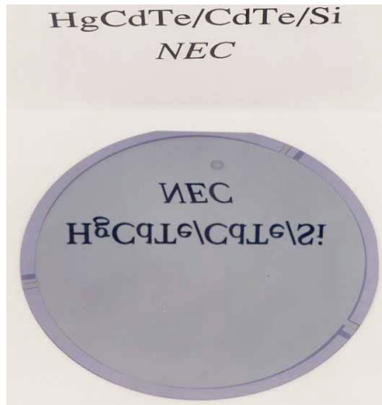
MBE grown HgCdTe surface on 3 inch Si wafer. Mirror-like surface morphology was obtained.
